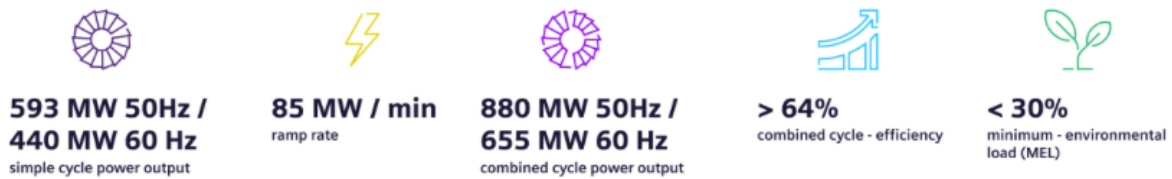
Figure 20: The "vital numbers" for Siemens Energy's fast-ramping combustion turbine (Source: Siemens Energy)
